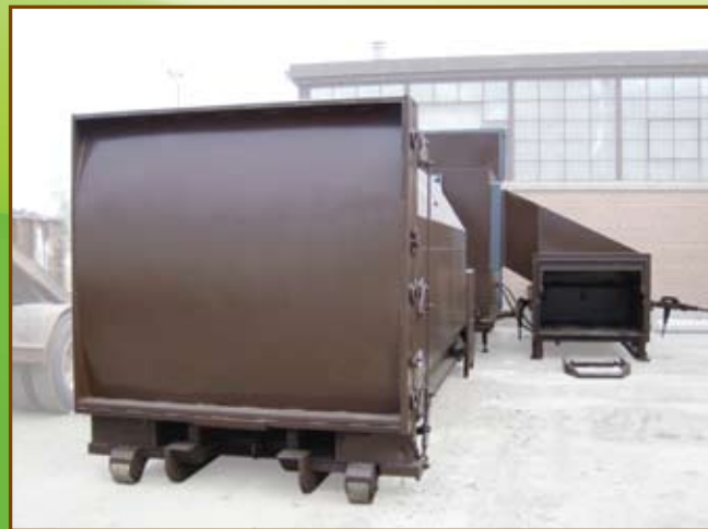
Weather Enclosure with Side Chute
